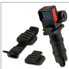
Standard Picatinny mount doubles as handheld for nighttime searching
