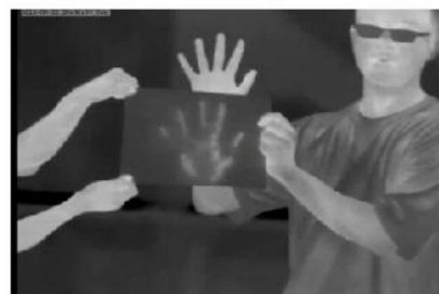
Residual heat detection
